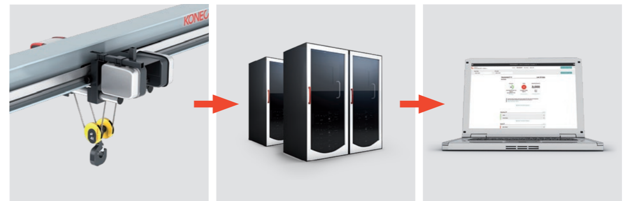
Sensors gather usage data - running time, motor starts, work cycles and brake condition.
