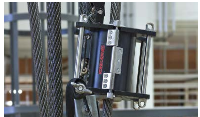
RopeQ detects internal broken wires that are not visible to the eye and would be missed by traditional inspection methods.
