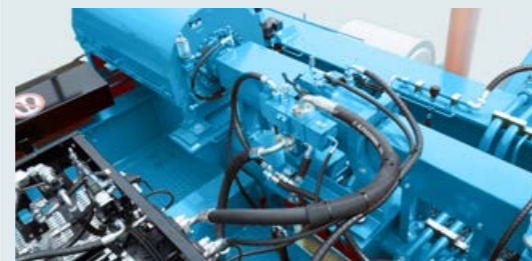
High-performance hydraulic hoist motor
