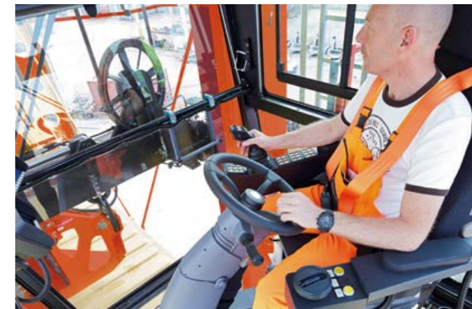
A cab that drivers like to work in: adjustable steering columns; electrically rotatable driver seat, on request; adjustable pedals
