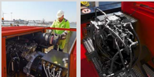
High-performance diesel-generator set with sliding cover for easy access. Ancillary hydraulics module supplies spreader, steering cylinders and brake system.
