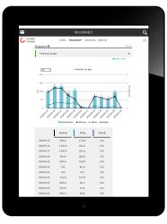
The **Alerts** section highlights safety critical alerts and production critical alerts. It also provides a Pareto analysis that displays and ranks the most important causes of alerts related to safety and the usability of the crane.
